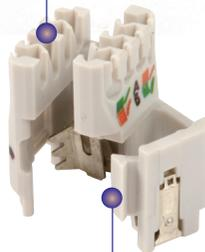
**Hinged Cable Retention** — Eliminates need to feed cable and conductors through an opening and can be closed manually or with the Z-Plug tool to accommodate multiple cable diameters (22-26 AWG). Also features dual grounding clips for shielded cables.
