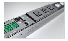
Easy to use and access, Smart PDUs from Server Technology offer input current monitors on easy-to-view LED via network or serial connection. These PDUs feature branch circuit protection and are available in a variety of voltages, amperages. Available in single- and three-phase.
